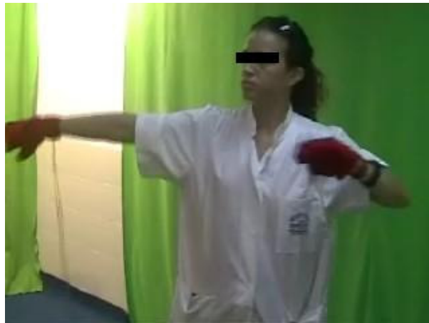
Figure 3: Subject wearing two red gloves with embedded vibrators on palmar surface and heart rate monitor
